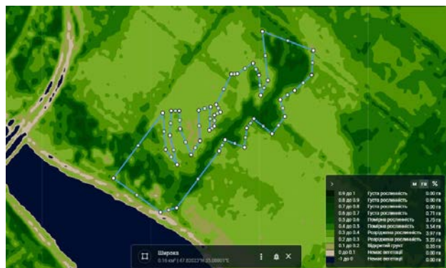
Fig. 3. Vegetation density of the Shyroka gully, determined using the NDVI vegetation index
